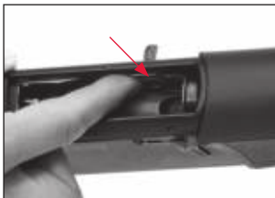
Push inward on the shell stop to unload the magazine.
