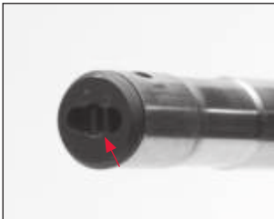
The three-shot adaptor shown secured in the magazine tube.
